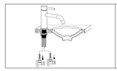
Connect the hot and cold flexible hoses to the isolation valves (not included), hot on the left, cold on the right.
