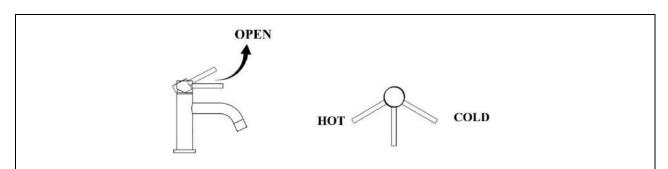
By lifting the Lever Handle upwards, the valve will be activated. Water flow will increase by continuing to lift up the Lever Handle. By rotating the Lever Handle counter-clockwise, the water temperature will decrease. By rotating the Lever Handle clockwise, the water temperature will increase.
